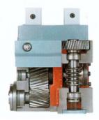
The gearboxes of the VMS machines are exceptionally rigid. The sawblade spindle, the intermediate shaft, as well as the worm gear are all hardened and ground to ensure exceptionally long life. Combined with the patented "Eisele Torque Equalizer" these gearboxes will provide the smoothest, fastest cut, for the longest time.
