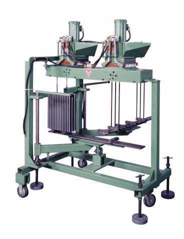
The Tridan Model **VC-2SM-10-48 Vacuum Fin Collector** Is designed as a complete single blower vacuum system for the automatic collection of heat exchanger fins as they progress from a die. The completed fins can be removed by manually swinging the collector arms into alternation positions on either side of the fin collector frame.
