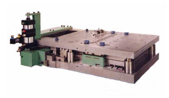
The Tridan Model **RDVS Superform Ribbon-Typle Fin Die with Self-Contained Pull Feed System and Integral Feed Progression Changer.** The production application of this die is to progressively form collared holes with a specific inside diameter and height, in a prescribed geometric pattern, and from a designated fin stock material, alloy, and thickness range.
