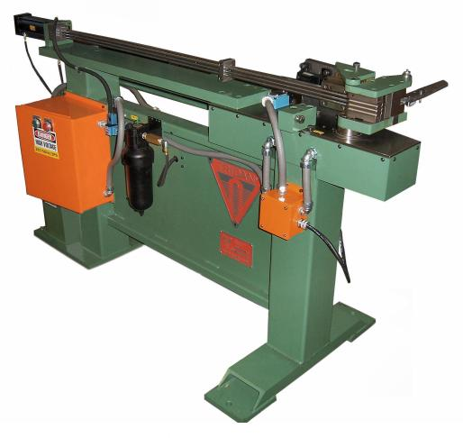
The Tridan **Hand Fed Power Assist Hairpin Bender** is designed for the production of hairpin benders from straight pre-cut lengths of copper or aluminum tubing. Upon manual feed and clamping of the tubes, the HBPA then performs the bend with the assistance of a hydraulic cylinder.
