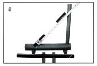
Place the PipeMaster on the opposite stub with the indicator mark over the centerline. Adjust the pins to fit the joint. Measure the distance from the housing to the mark on the first stub.
