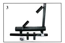
Place the PipeMaster on the pipe to be cut. Align the housing with the centerline. Mark the location of the housing on the pipe and trace the shape of the cut line.
