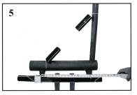
Transfer the distance measured in step 4 to the pipe to be cut. Place the PipeMaster on the pipe at this location and align the centerlines and mark the cut line.
