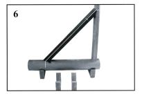
Remove stubs and grind tack welds. Check final fit and weld in place.
