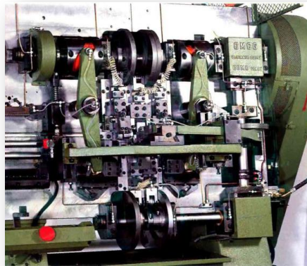
Bending and forming area detail
