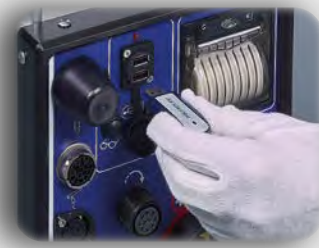
USB memory stick for saving, loading and archiving of welding programs and monitored welding data
