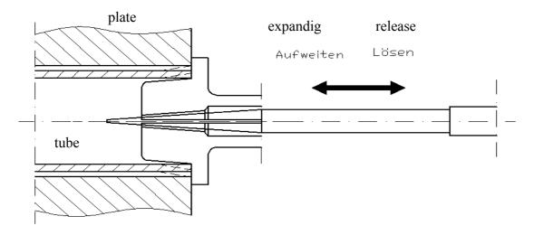
The expanding cylinder is acted upon by the hydraulic unit by means of oil pressure, and the piston of the spreader cylinder moves out.
