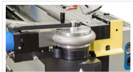
The TUBOMAT's bending head with the optimized tooling concept.
