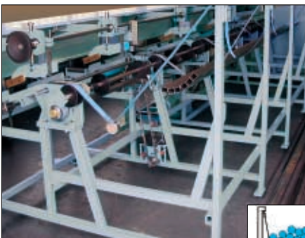
Bundle loading magazine for the automatic loading of round, rectangular and square material with separation unit for thinner cross sections.
