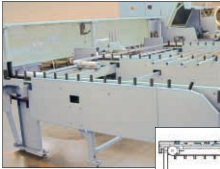
Flat magazine (chain) for automatic loading of all profiles.
