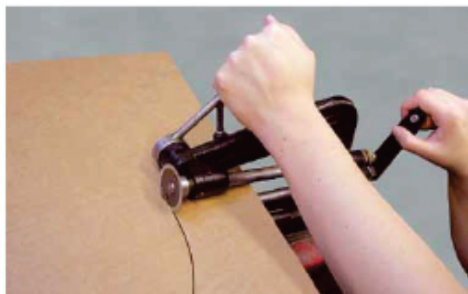
(Figure 7) Turn the hand crank clockwise. Simultaneously, with the other hand, maintain a constant downward pressure on the cutting disc lever. As the cutting discs rotate, the gasket material will be drawn towards the cutting discs initiating the cutting process. Continue cranking until the entire OD of the gasket material has been cut. Disengage the top cutting disc. Discard unwanted material.
