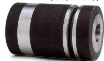
Combination Rollers urethane midsection/ heat-treated steel hub for all around performance when a mar-free finish cut and steel backup is required for heavier (14 gauge and up) chrome-plated stock.
