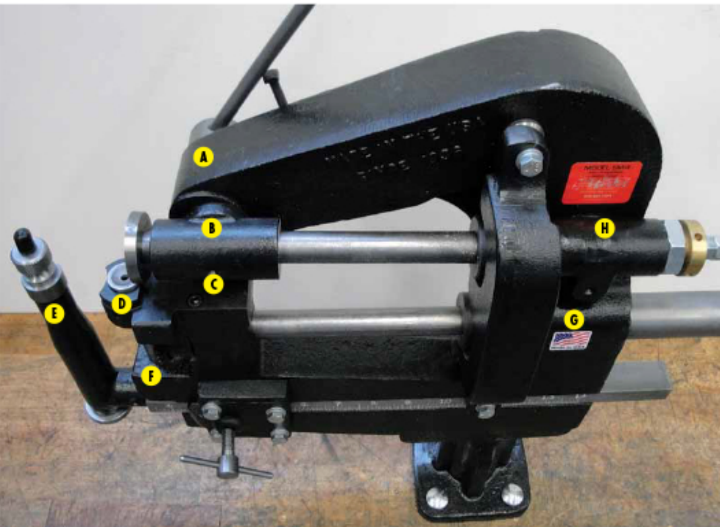
(Figure 17) The Model SM4 is pre-lubricated at the factory. Like any piece of precision machinery, regular cleaning and lubrication of all gears, and moving parts is recommended. Light machine oil should periodically be applied to points A, B, C, D, E, F, G, and H. Replace worn parts as necessary.
