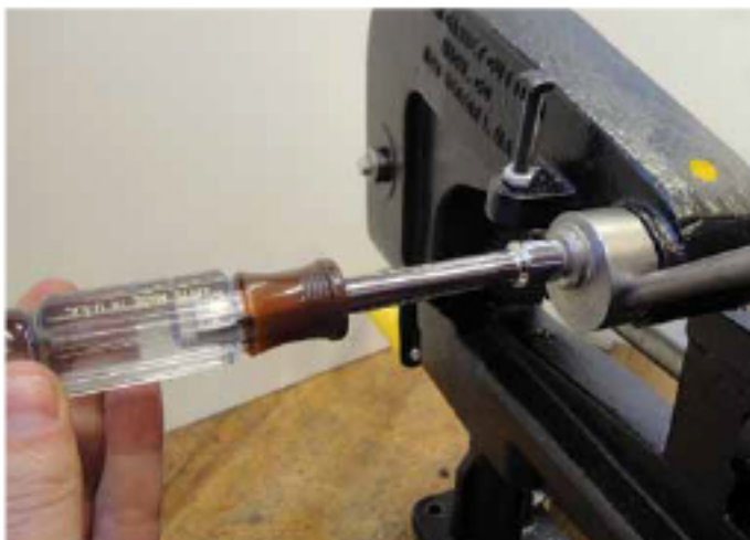
(Figure 10C) Remove the top shaft assembly by first removing the hex cap screws which hold the top cutter lifter bearing ( Figure 10C ) and thrust bearing housing ( Figure 10D ) in place using 7/16" wrench.
