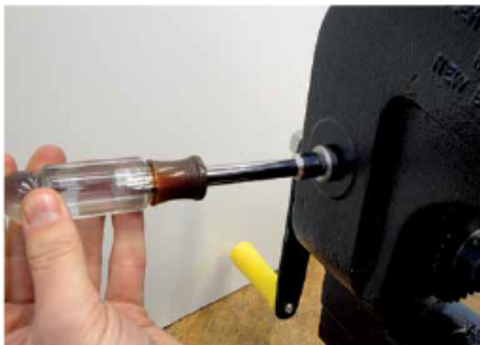
(Figure 10C) Remove the top shaft assembly by first removing the hex cap screws which hold the top cutter lifter bearing ( Figure 10C ) and thrust bearing housing ( Figure 10D ) in place using 7/16" wrench.
