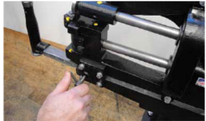
(Figure 3) Loosen the scale bar T-screw and slide the scale bar to the desired OD setting. Hand tighten the T-screw.
