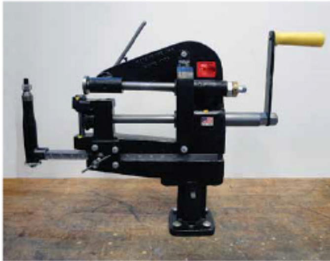
(Figure 1) Model SM4 is a heavy-duty unit and is typically bolted to the flat surface of a workbench using the four 3/8" diameter holes on the mounting base.
