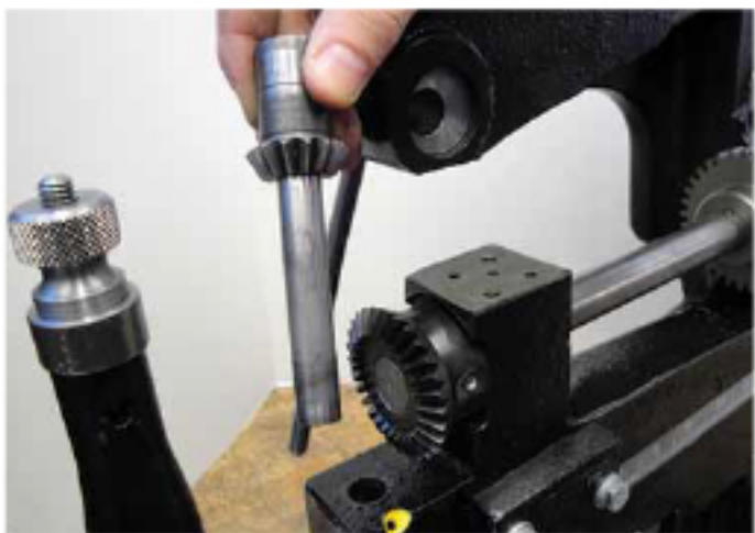
(Figure 10F) Lift bottom cutter out of frame assembly.
