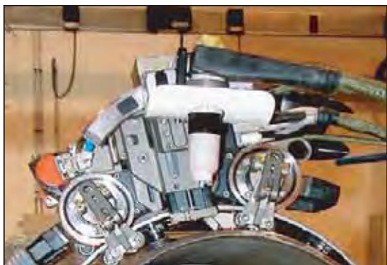
Front view of the carriage with the dynamic inclination module
