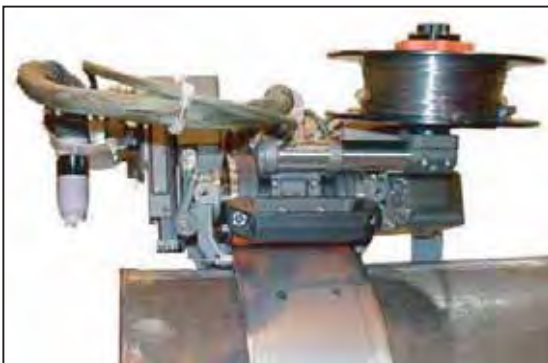
Side view showing the macro connector on the right
